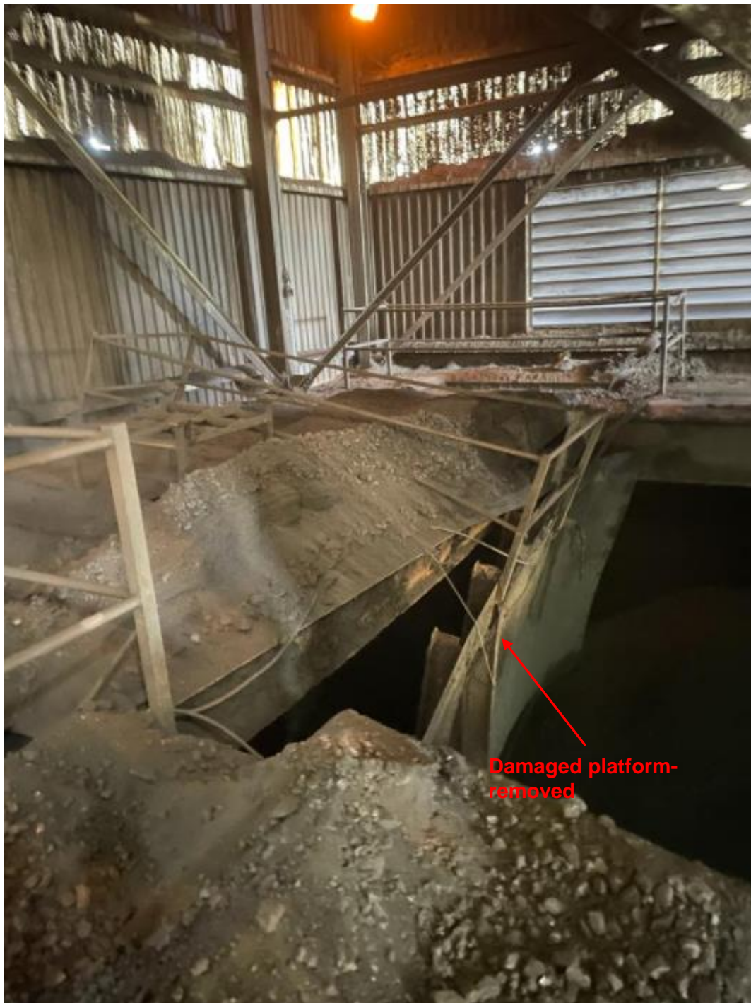
Figure 2: Damaged Platform hanging into Surge Bin hopper
